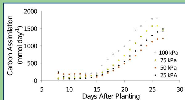
Figure 3. Whole canopy carbon assimilation of lettuce at various total pressures (25-100 kPa) over a 28 day period.
