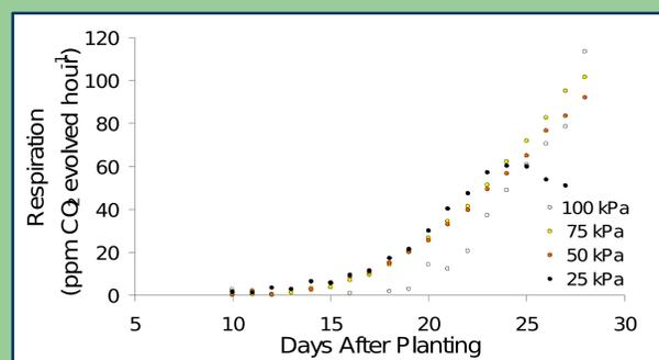
Figure 4. Respiration of a lettuce canopy at various total pressures (25-100 kPa) over a 28 day period.
