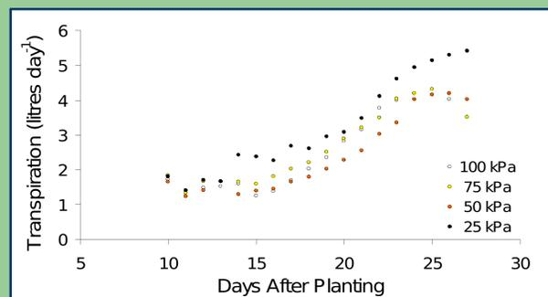
Figure 2. Whole canopy transpiration rates of lettuce at various total pressures (25-100 kPa) over a 28 day period .
